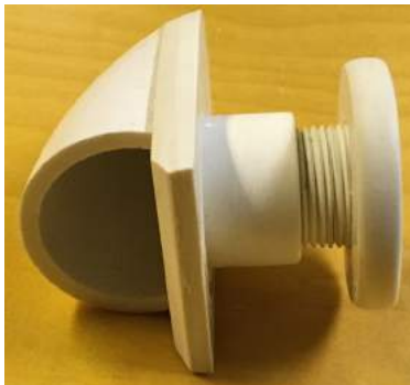
Housing and cap finished; all pieces made of PVC
