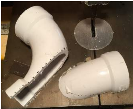
Cutting the elbow on the band saw
