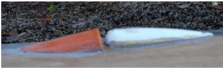
Scupper bailer and bullet made of PVC pipe
