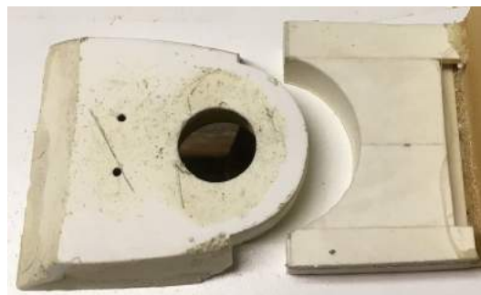
Glued PVC stack ready to glue to housing
