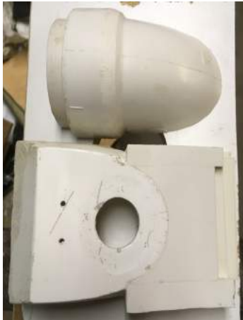
Elbow ready for gluing to bailer housing
