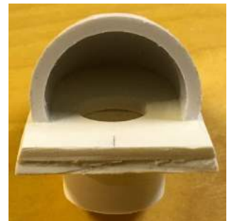
PVC sheet (from 2" Schedule 40 pipe); top of a 1-1/2" 90° PVC elbow; 3/4" NPT threaded PVC adapters
